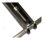
Weight rod showing slot for thumbscrews and fine balance weight
