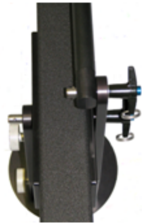
6. Fulcrum from above note parallel rod and connector pin placement
