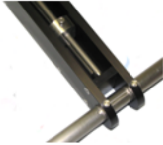
9. Weightrod showing slot for thumbscrews and fine balance weight
